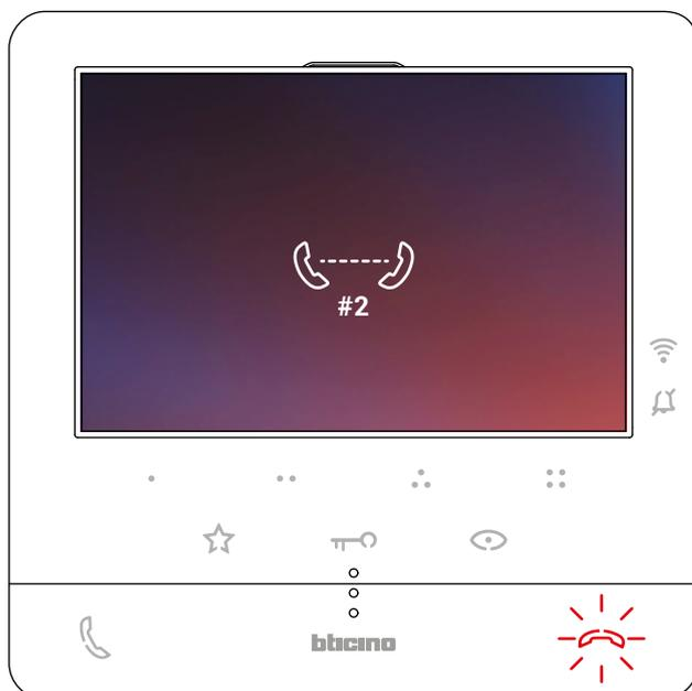
When the Internal Unit answers, the key starts flashing. Touch it to end the call or establish communication with the Internal Unit.
