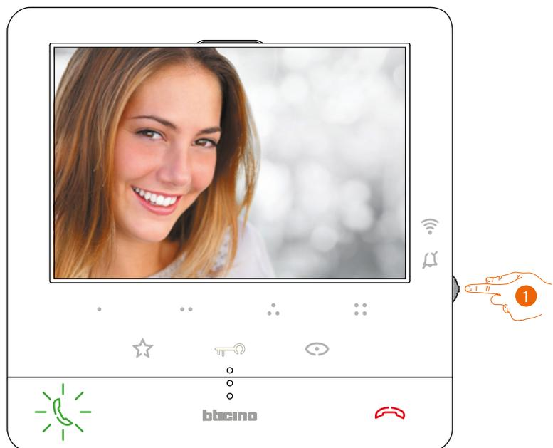
1. If necessary, during the call press the joystick to display the image sound/brightness/contrast/colour adjustment menu (see [Audio/video parameter adjustment](#)).
