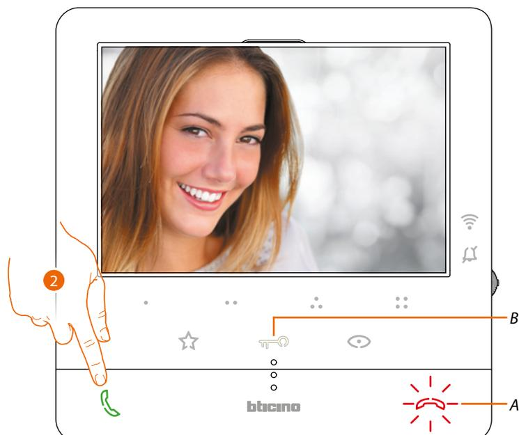
2. Touch to answer the call. The LED switches off. To end the call touch the (A) key, and to open the Entrance Panel door lock touch the (B) key.
