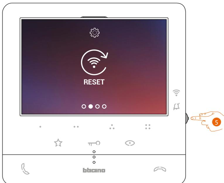
5. Press the Joystick to reset the Wi-Fi network and connect Classe100 X16E to another network, or to the same network with a different password.
