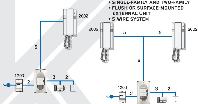
Style Kit 5 is the "ideal" door entry phone kit which uses 5 wires and is available in the single-family and two-family version. Style Kit 5 has an original and innovative design characterised by its unmistakeable and exclusive blue LEDs, by large name labels and by high sound quality. Simply by adding a telephone or an additional bell allows easy expansion and an elegant desk base ensures flexibility for all needs.
