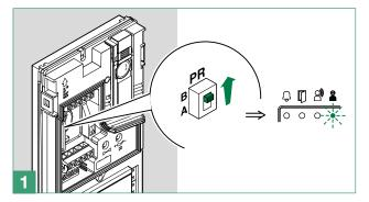
Set the DIP-switches to position 206 (ON 2,3,4,7,8) in accordance with the addressing table
