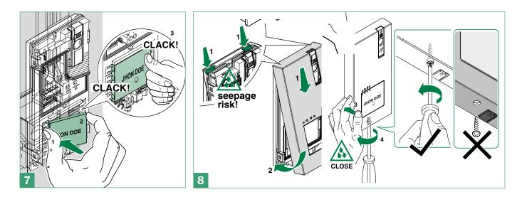
To ensure that the product remains water-tight, make sure that the fixing procedure is carried out correctly.
