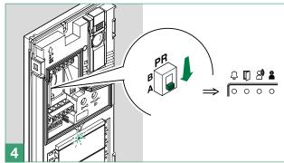
Reset the configuration of the DIP-switches
