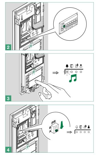
Reset the configuration of the DIP-switches.
