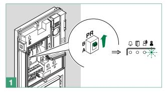
Set the user code using the DIP-switches in accordance with the addressing table
