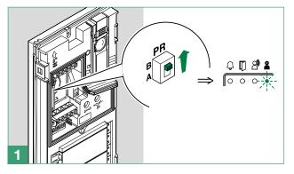
On the DIP-switch, set the code corresponding to the function you want to program as shown in the table.
