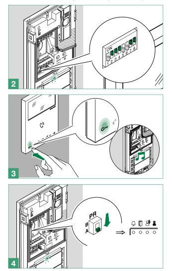
Reset the configuration of the DIP-switches.
