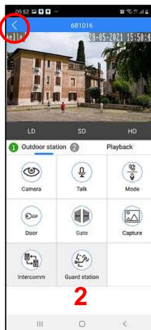
If "VIDEO BUSY" appears on the display after a camera request from the app, it means that a connection is already in progress between the outdoor station and an apartment video door phone or between the outdoor station and another smartphone.
